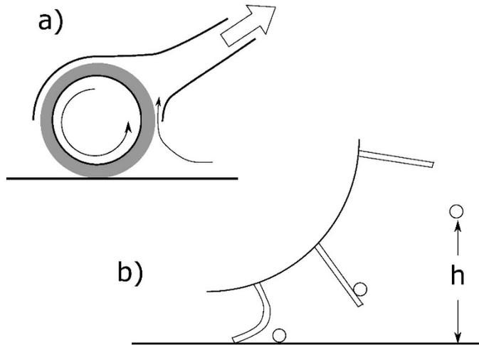
Part (a) of the figure is a generic sketch of a vacuum cleaner brush. Air is sucked between the brush and the housing to entrain dirt particles which are then carried to the filter. The bristles, here indicated by shading, agitate the dirt and lift it into the air stream.
